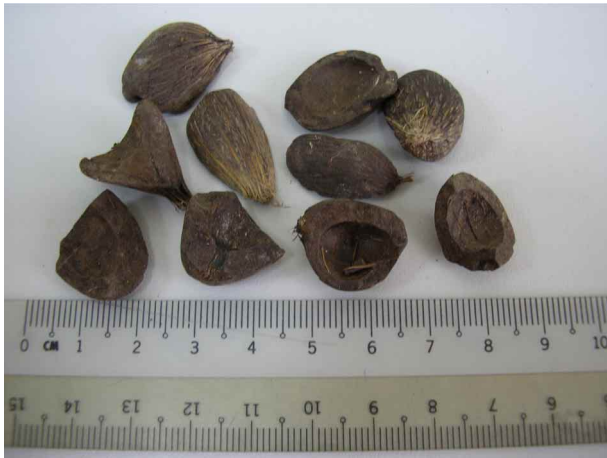
Figure 3. Various shapes of OPS aggregate.
