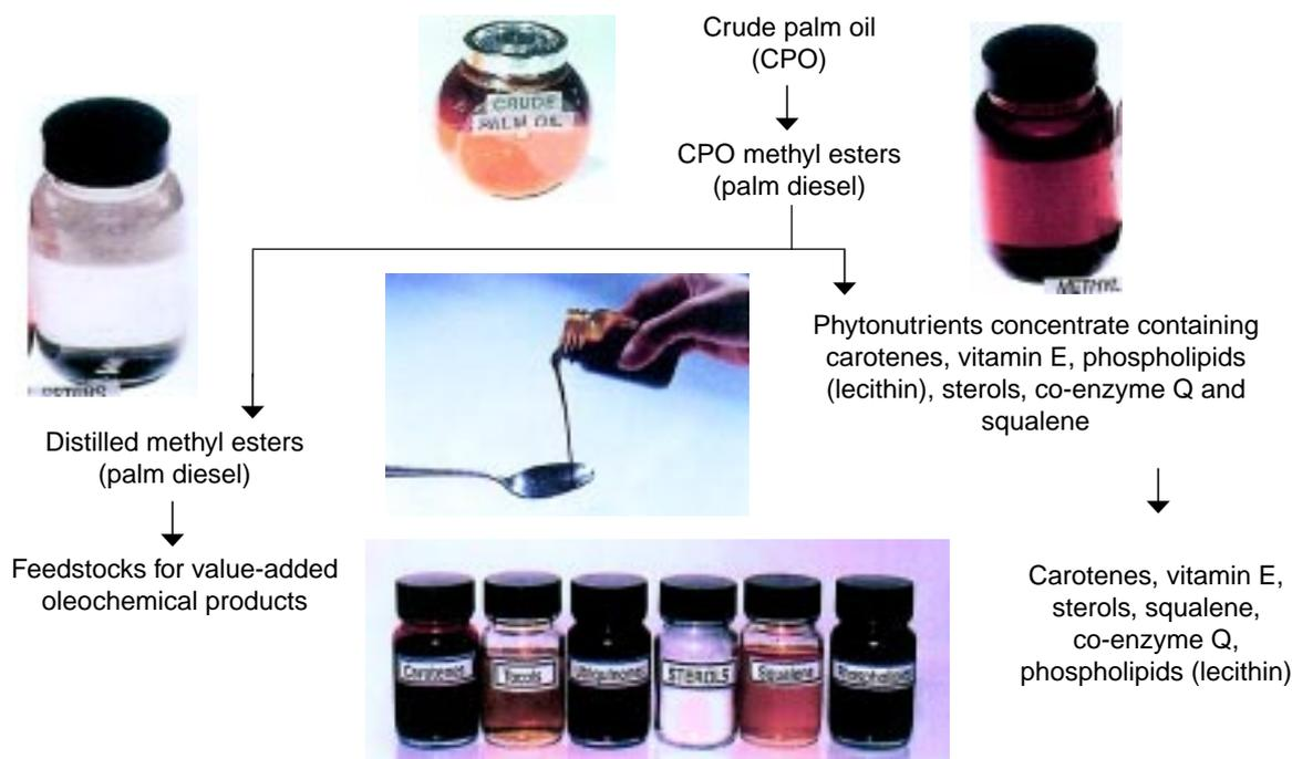
Figure 3. Integrated process for production of palm diesel and palm phytonutrients.
