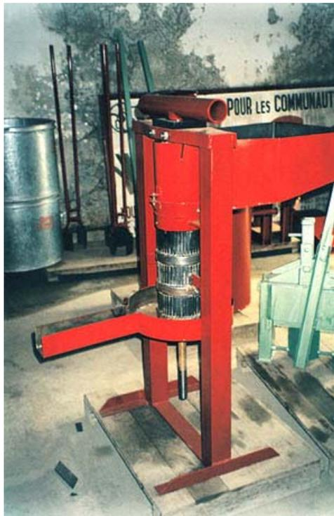
**Fig. 10 Motorised horizontal screw press (Centre Songhai, Benin)**
