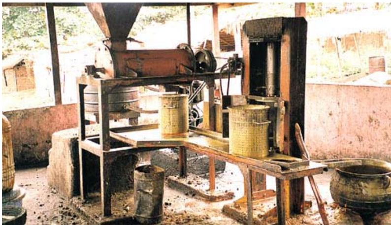
**Fig. 12 Flushing extractor (Cort Engineering Services, Ghana)**
