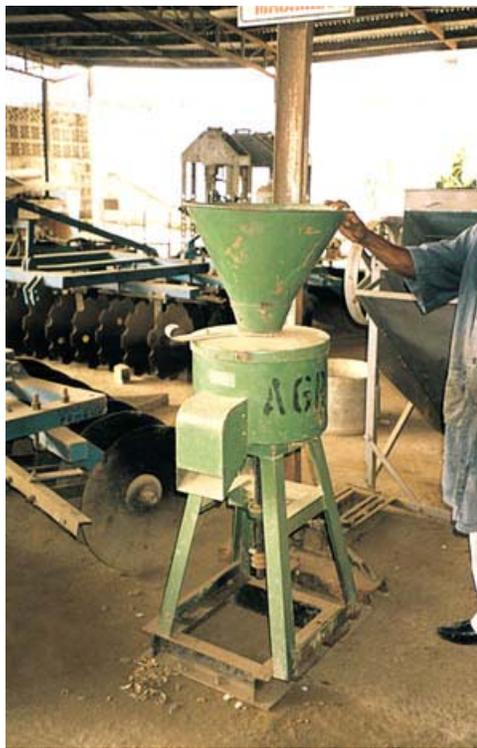
**Fig. 17 Palm nut cracker (NOVA, Technologies, Nigeria)**
