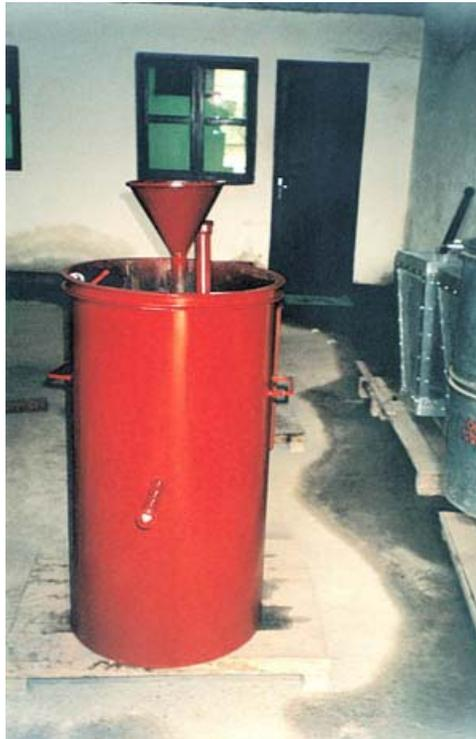
**Fig. 14 Clarifier tank (Nova Technologies Ltd., Nigeria)**
