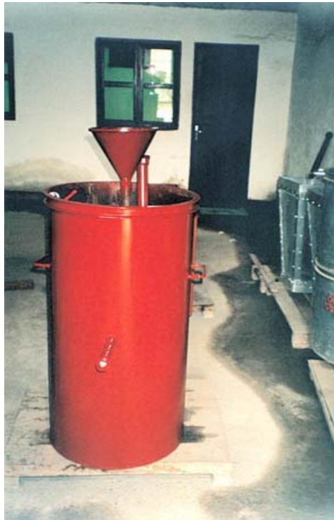
Fig. 14 Clarifier tank (Nova Technologies Ltd., Nigeria)
