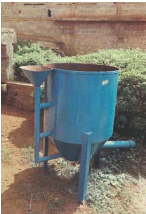
**Fig. 14 Clarifier tank (Nova Technologies Ltd, Nigeria)**
