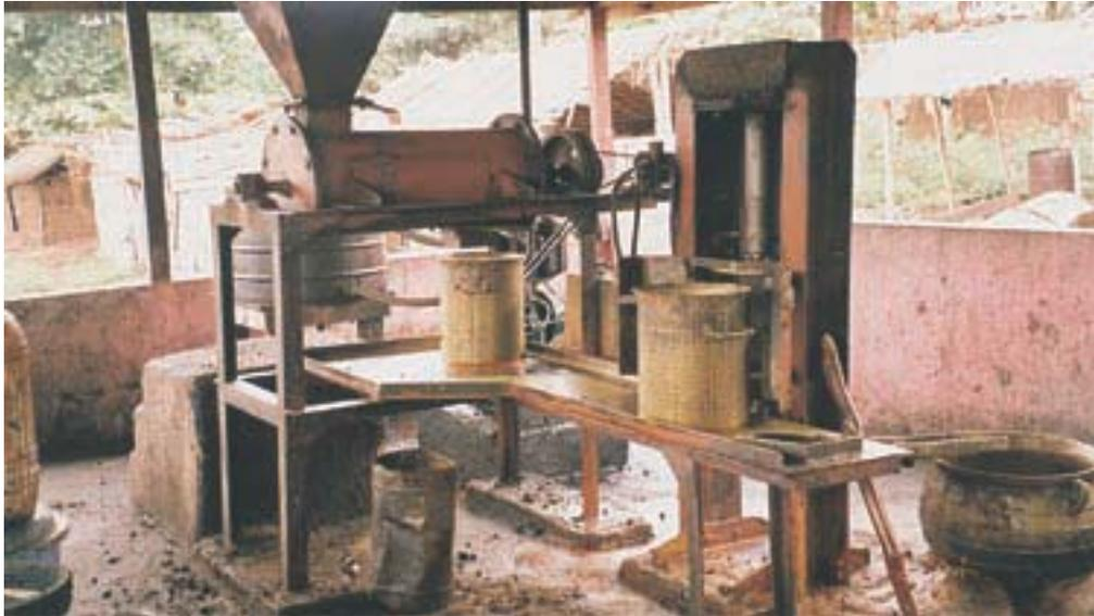
**Fig. 11 Combined digester and motorised hydraulic press
