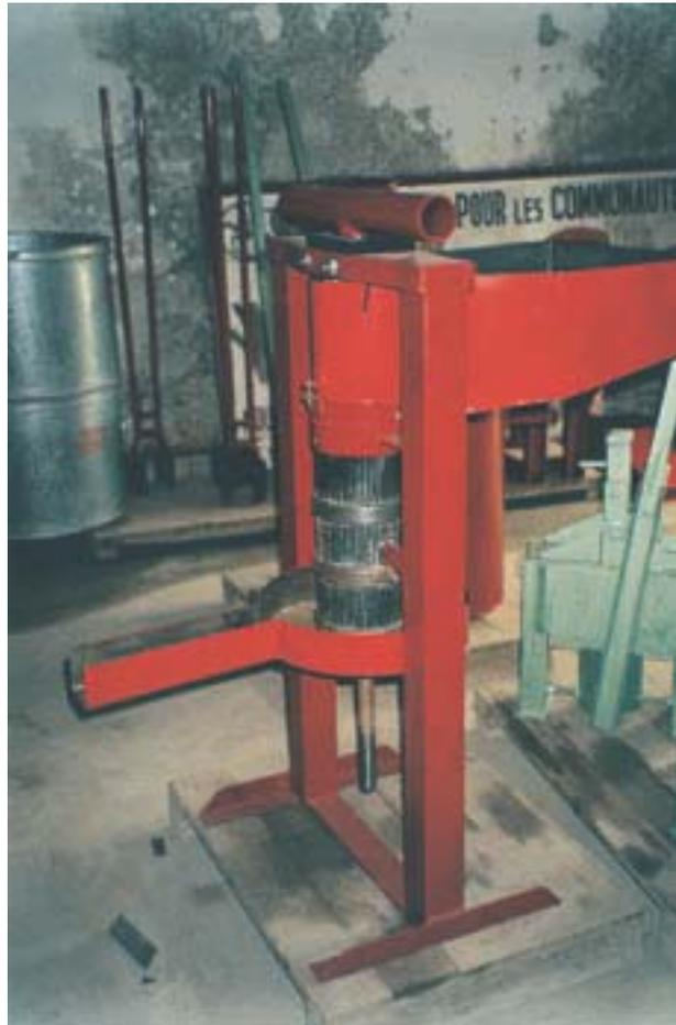
**Fig.9 Manual vertical press (O.P.C., Cameroon)**
