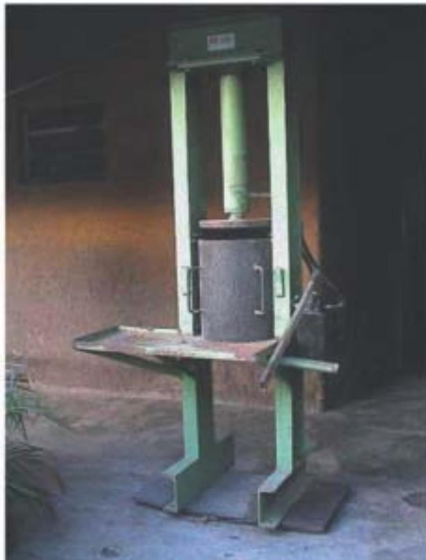
**Fig. 8** Hydraulic press (manual)
