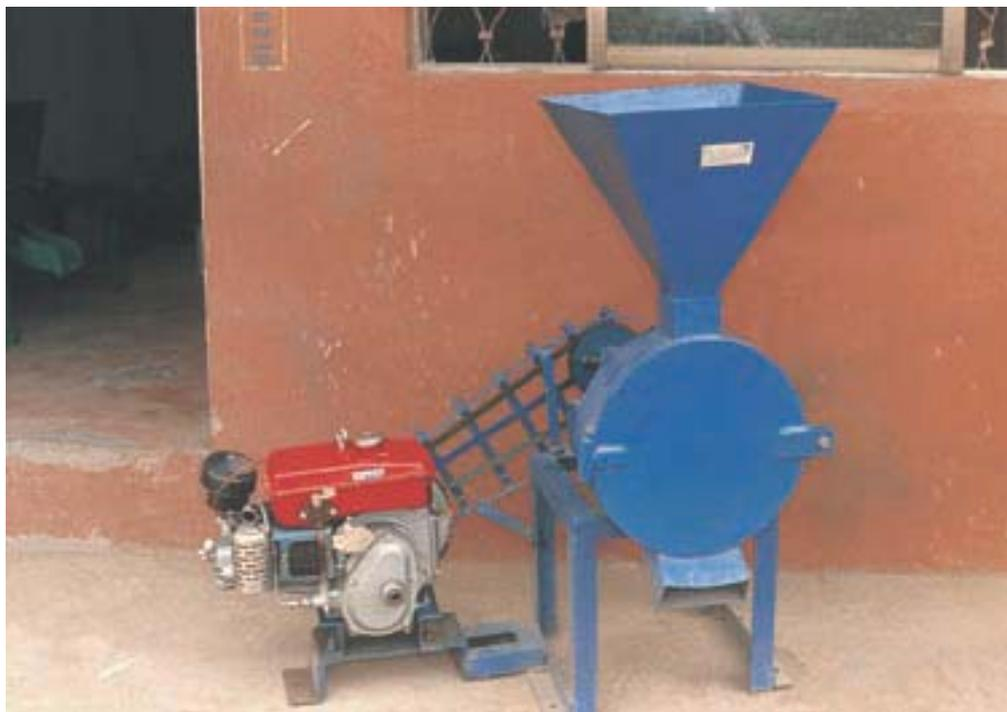
**Fig. 17 Palm nut cracker (NOVA, Technologies, Nigeria)**
