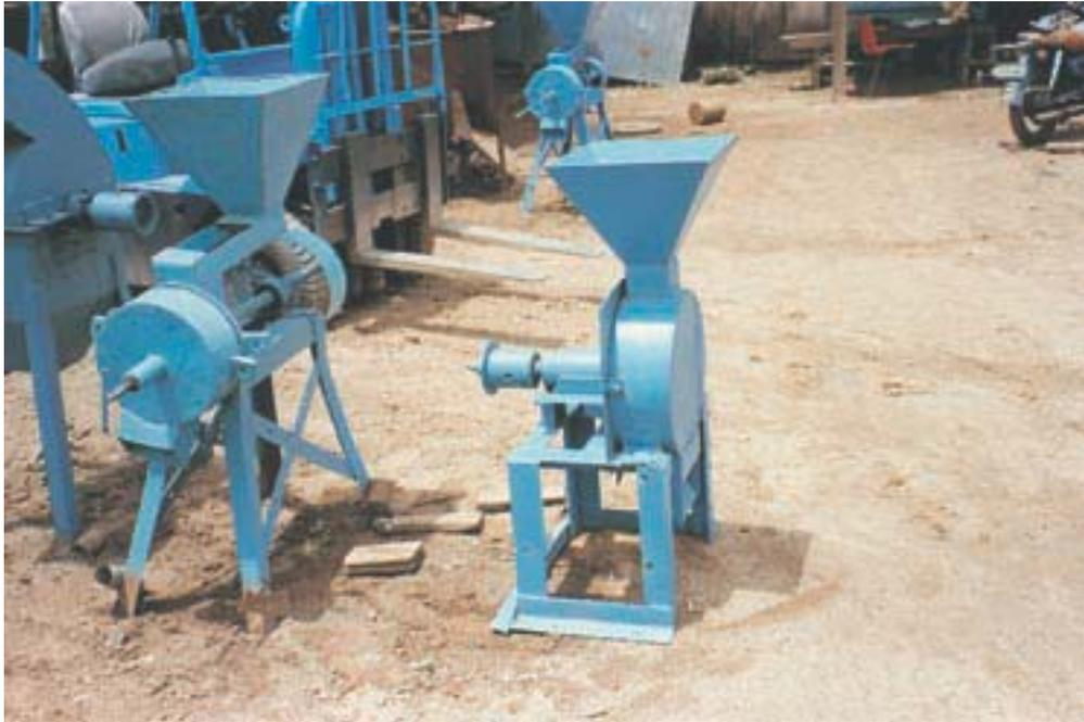
**Fig. 18 Palm nut cracker
