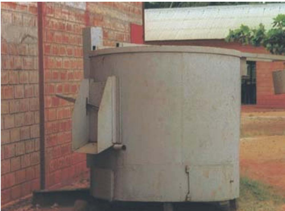
**Fig. 4 Fruit sterilizer (Centre de Formation Technique Steinmetz-Benin)**
