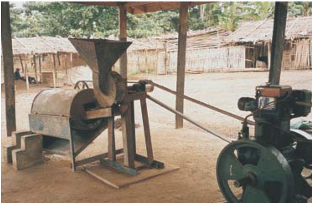
**Fig. 19 Palm nut cracker combined with Kernel/Shell separator
