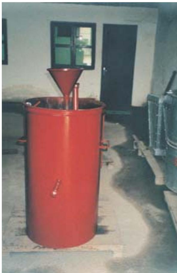
**Fig. 13. Clarifier tank (O.P.C., Cameroon)**
