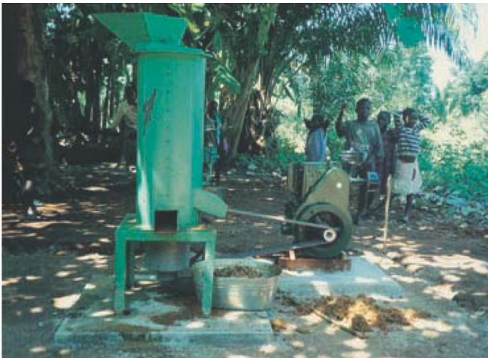
**Fig. 12 Flushing extractor (Cort Engineering Services, Ghana)**
