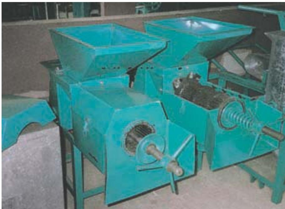
**Fig.10 Motorised horizontal screw press (Centre Songhai, Benin)**
