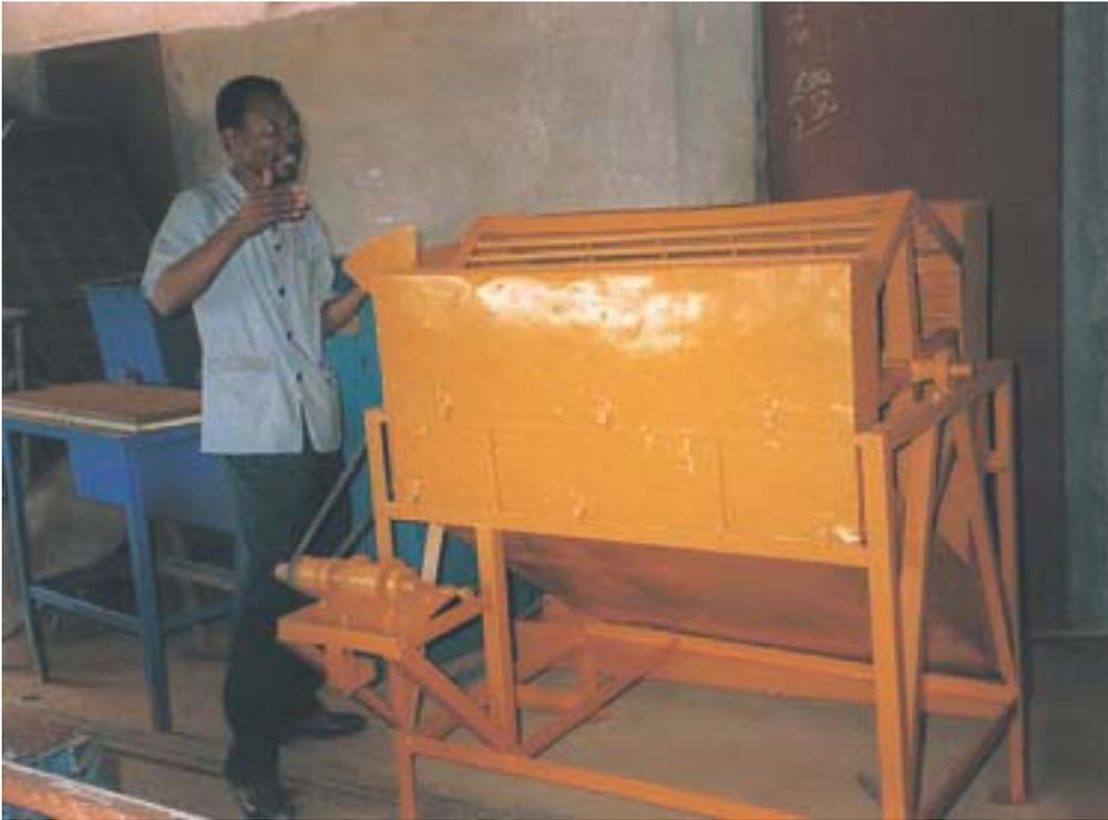
**Fig. 3 Bunch thresher (Centre de Formation Technique Steinmetz-Benin)**
